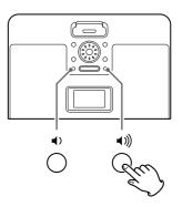
The volume can be adjusted from Muted (00) to Max (20). To reduce or turn up the volume continuously, hold down the Volume button (◆ or ◆)).
